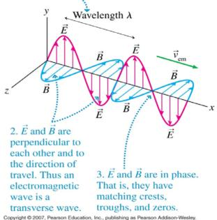
(b) Right-hand rule for electromagnetic waves
