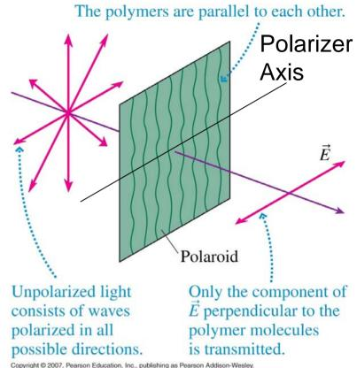
Only the electric field component parallel to the polarizer axis is transmitted. The perpendicular component is absorbed. Since all possible polarization directions are represented in unpolarized light, 50% of *unpolarized* light is transmitted <sub>9</sub> by a polarizing filter and 50% is absorbed.
