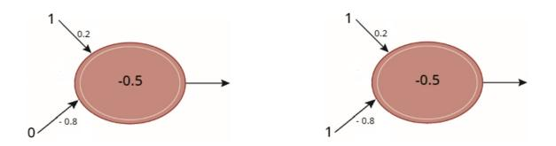
The first perceptron has a sum of 0.2 which exceeds the threshold weight of -0.5, so it will have an output of 1.
